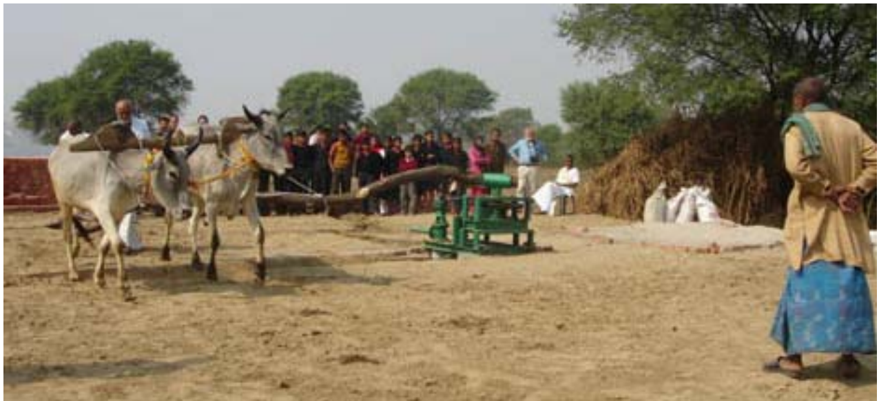
Two Amrit Sagar bullocks powering an innovative pump that can be used to pump well water as well as grind crops (photo by Kamla).
